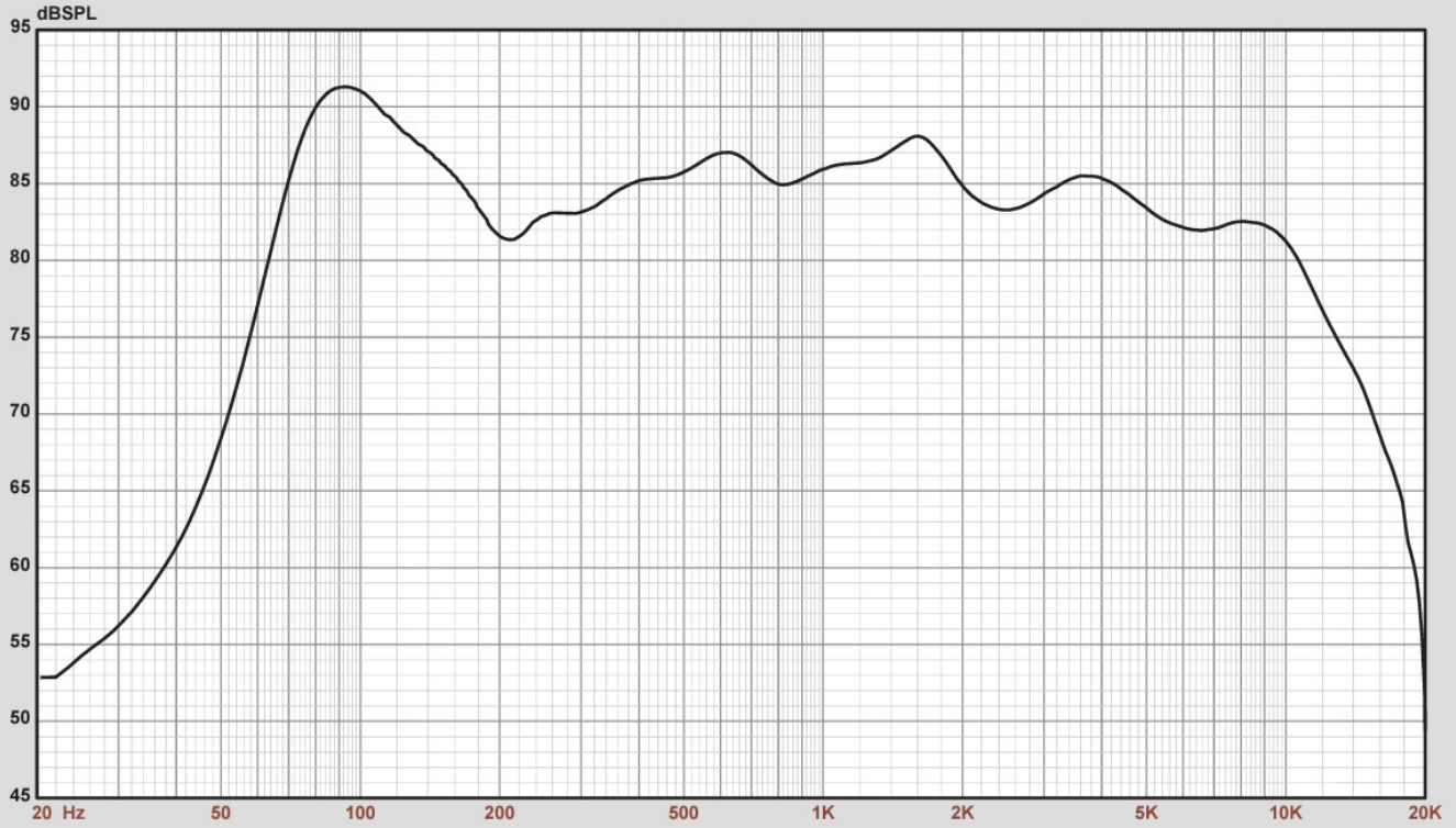
LookHear Frequency Response with 2.83V at a 4m (13.1 ft) distance and at a listening position of 1.7m (5.5 ft) high with DSP applied.
